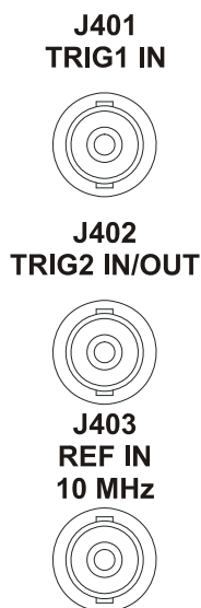
Figure 1-10: Trigger and Reference Connectors
